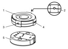
Figure 2 PROG Key and IR Port of ZXT-120
